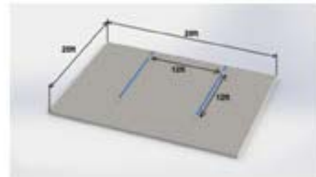
4 Standard Power Outlets in the Floor
