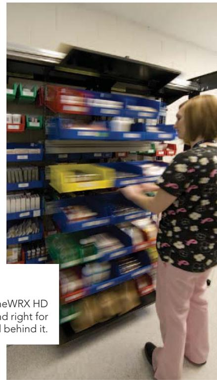
The front section of the FrameWRX HD system slides to the left and right for access to materials stored behind it.
