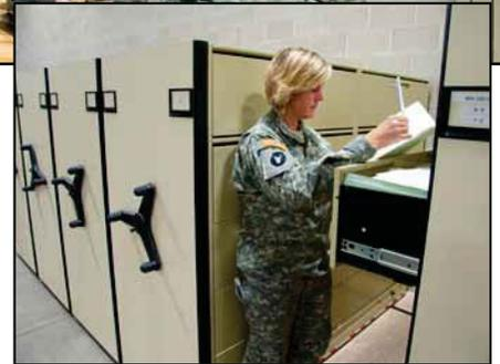
Archived files take up significantly less floor space when compacted using mechanical assist mobile carriages but provide quick and direct access.
