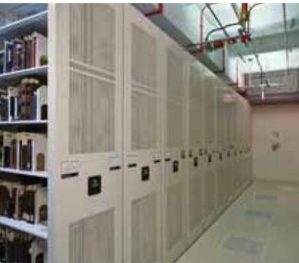
With perforated end-panels and other components, the powered HDMS system facilitates air circulation – even when mobile carriages that house materials are closed and not in use.
