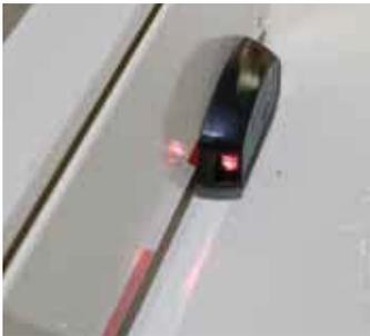
An infrared light beam is projected along the length of each carriage at the base to stop carriage movement when the light beam is broken, preventing carriages from contacting a person or an object.
