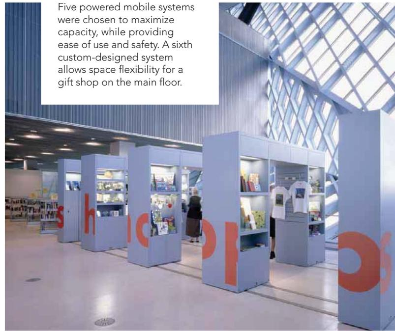
Five powered mobile systems were chosen to maximize capacity, while providing ease of use and safety. A sixth custom-designed system allows space flexibility for a gift shop on the main floor.
