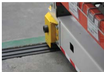
Recessed rails on the ActivRAC system create a smooth surface for forklift travel.
