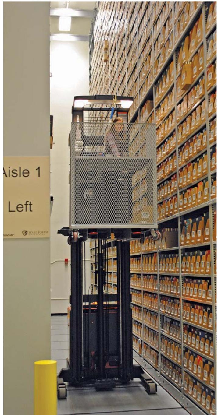
Integrated guide wire: when the bays open up and give someone access to the aisle, the forklift is centered on a guide wire, which keeps it on course. This means a user cannot run off course and into the shelving system.
